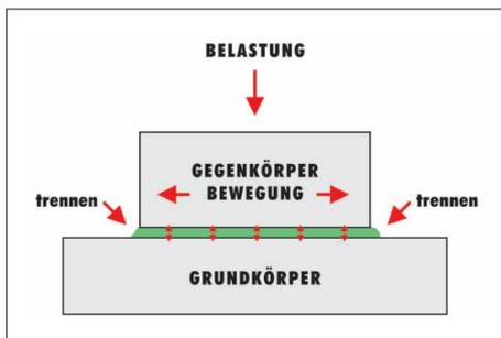
Despite a high pressure load and the shearing movement of the base body, the lubricating film of the HHS 2000 remains active and does not pull away. Reliably separates counter body from main body, thus ensuring optimum wear protection under high pressure loads. This is only possible with dirt-free lubricating points, which is why we recommend careful and thorough pre-cleaning with HHS Clean, Art. 0893 106 10, before each use.
