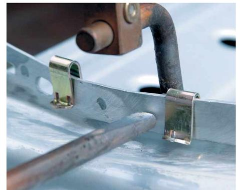
3. The powerful force of the fixing clamp keeps the clamped sheet metal in place. To remove the fixing clamp, slide the pliers over it and open the clamp.
