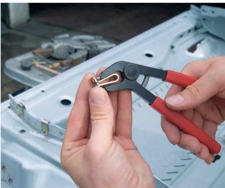
1. Insert the fixing clamp into the special pliers and open the clamp.
