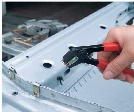
2. Slide the clamp over the sheet metal edges to be joined and release the pliers.
