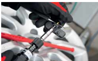
Fixing rubber valve on the sensor with 1.4 Nm
