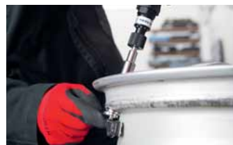
Tightening the union nut with 8.0 Nm on a metal valve
