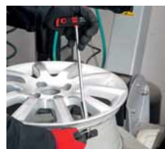
Removing metal valve
